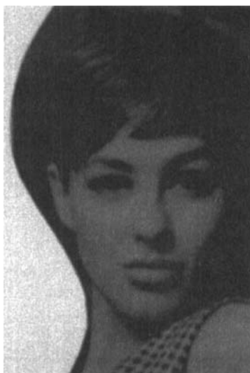
FIGURE 10 Photograph of a photo-aligned and photo-structured LPP/LCP dichroic guest-host linear polarizer image on a TAC film. The invisible part of the image on the left hand side of the picture is viewed in unpolarized light.
